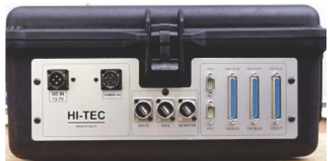
Above: NaviControl Control Unit in the manual gearshift configuration (Daq and CAN Bus connector side).
