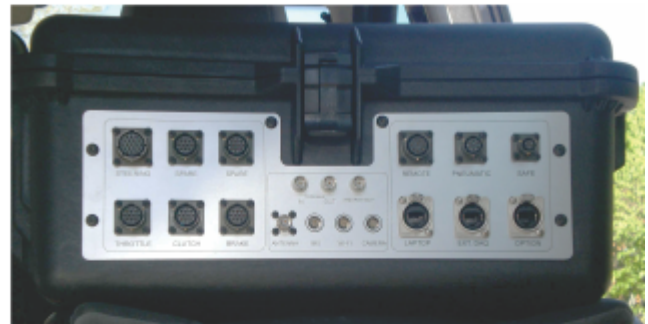
Above: NaviControl Control Unit in the manual gearshift configuration (robots connector side).
