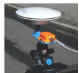
Bottom: on the left the Remote Joystick Unit, on the right the GPS antenna and the IMU fixed on the windshield.
